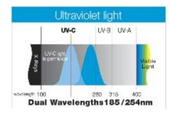
UVPhotoMAX™ uniquely uses two wavelengths of UV-C light to kill germs and destroy odors.
